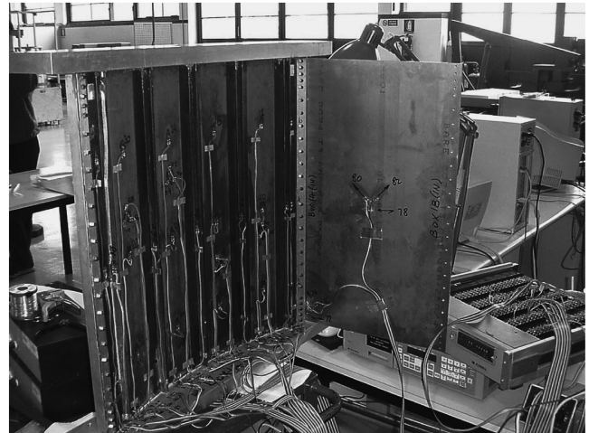
Fig. 6 Panel with a side aluminum plate and bonded strain gauges.
